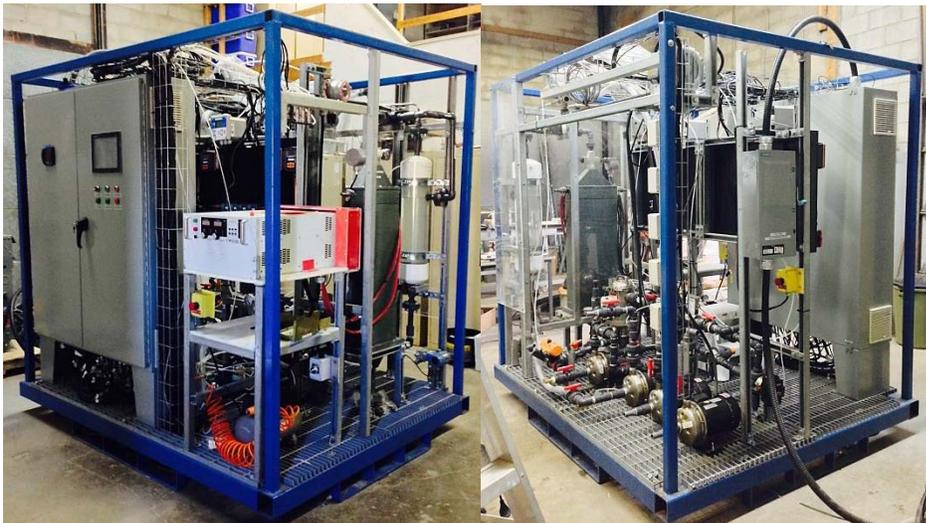
*The 1.0 gpm pilot-scale electro-oxidation leachate treatment system.*
